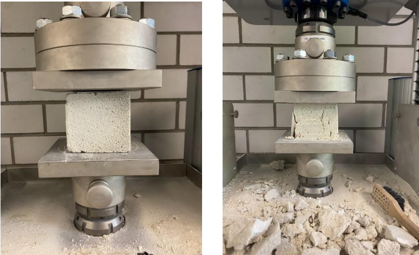
Figure 5.1.5 Compressive strength test of NRG foam.
