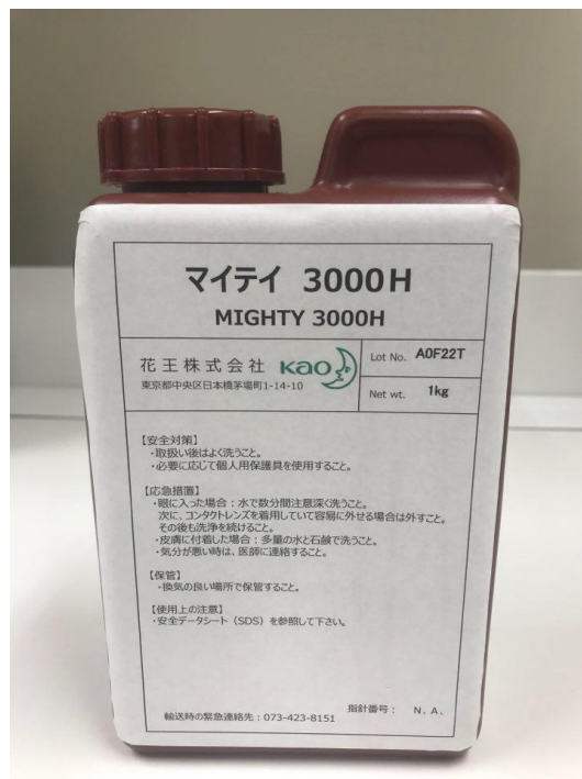
Figure 2.1.6 Superplasticizer used as water reducing agent
