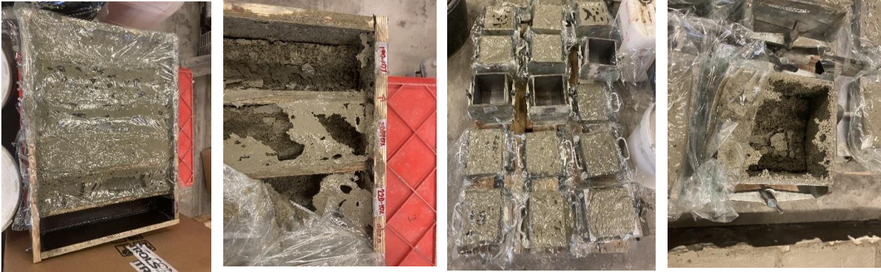
Figure 5.1.2 The mixtures of NRG foam with Nextek24 PCM with 10% collapsed foam structure.
