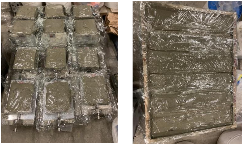
Figure 5.1.3 The mixtures of NRG foam with Nextek24 PCM with 10% after increasing accelerator.
