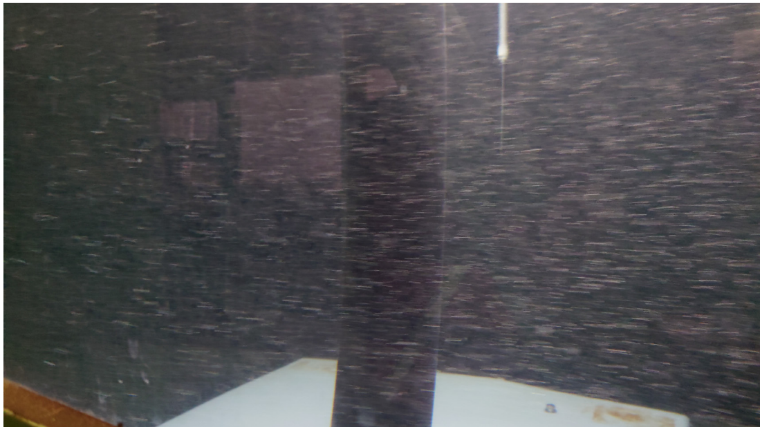
Fig. 4-10 Tracer particles filling the experimental water tank
