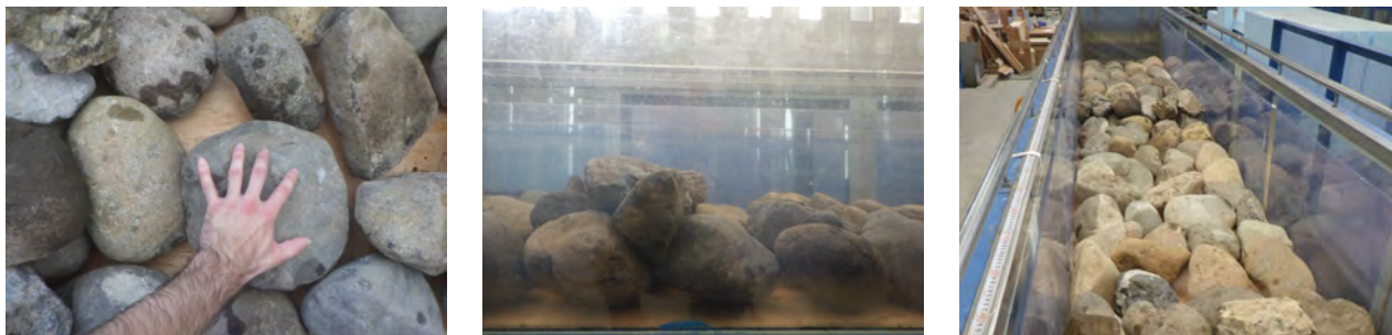
(a) Prototype-scaled boulders with the author’s hand for reference. (b) Side view of one of the ramps (left side wall). (c) The model is viewed from up-stream.
