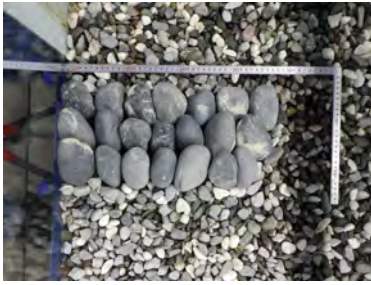
(a) Aerial view of one of the three boulders groynes.
