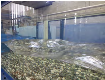
(a) Water surface above model GM1.3 for Q=0.155 m 3 /s.
