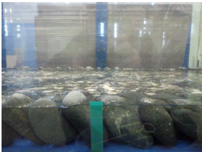
(a) Emerging gravel and boulders in model GM+AB1.
