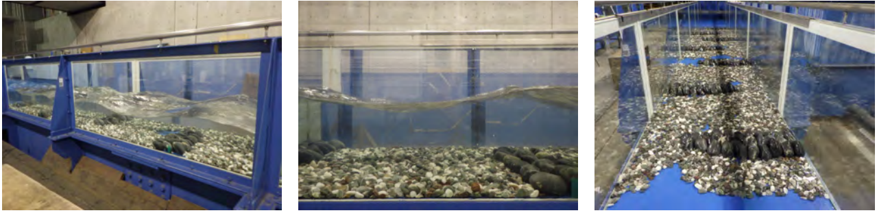
(a) Water surface above the model (flow direction right to left). Local erosion is visible in several areas. (b) Side view of the water surface (flow direction right to left). (c) The model after being exposed to Q=0.155 \text{ m}^3/\text{s} . Significant erosion is visible.
