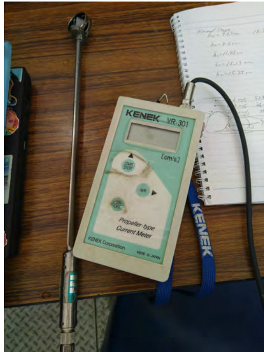
Figure 61: Propeller-type current meter KENEK Co. model VR-301.
