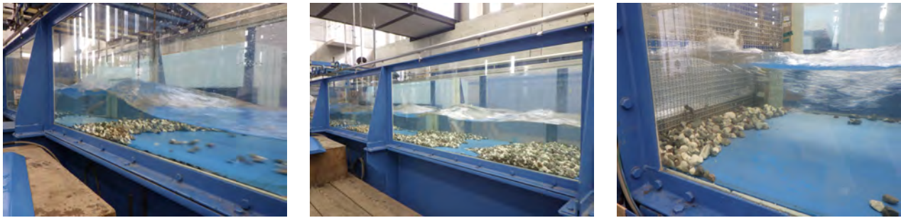
(a) Grains transport from one anti-dune to another.
