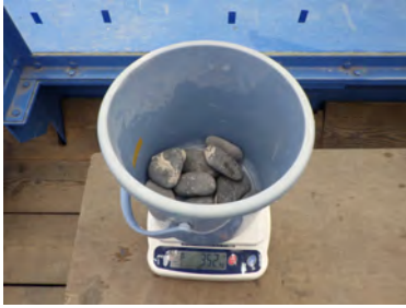
(d) A bucket full of boulders is weighed.
