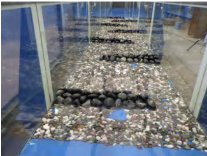
(a) Gravel erosion visible in model AB2.
