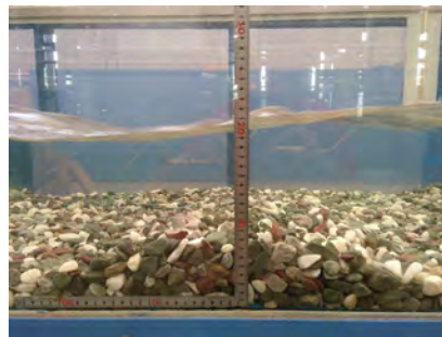
(b) Side view of the water surface above a gravel mount (model GM2.4) for Q=0.123 m 3 /s.
