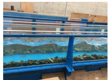
(c) The water profile at the downstream end of the model.
