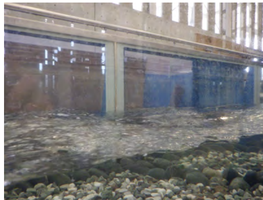
(e) Q=0.155 \text{ m}^3/\text{s} (failed experiment).
