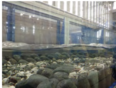
(b) Water surface profile over model GM+AB3.
