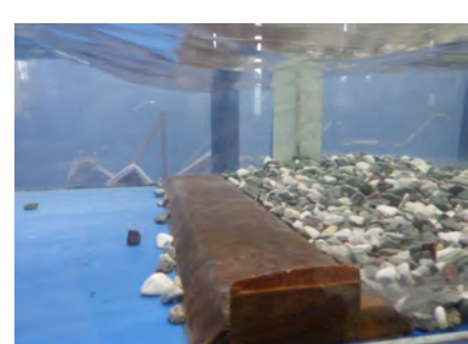
(c) Gravel eroded downstream for Q=0.155 m 3 /s (model GM1.3).
