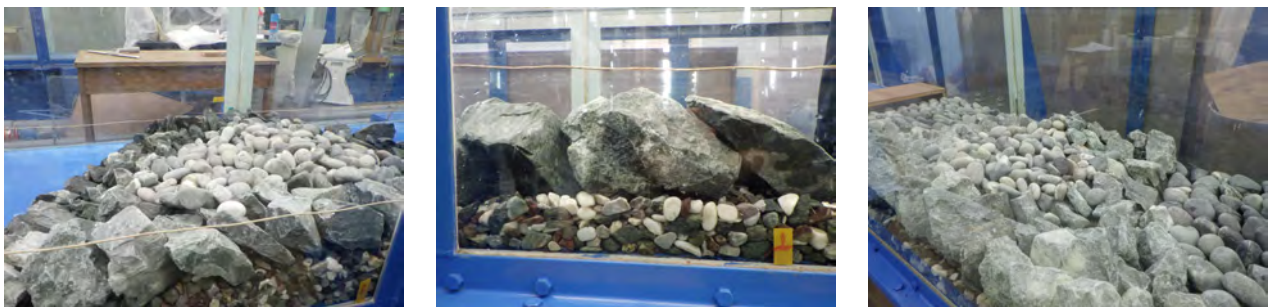
(a) Construction of one scaled gravel mount. (b) Composition of the assembled boulders along the side wall. (c) The completed model scaled 2.5 times viewed from upstream.
