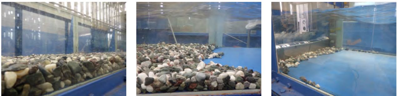
(a) Model set-up with 0.0400 m thick, flat gravel bed. (b) Upstream scouring in case of Q=0.143 m 3 /s. (c) Gravel erosion in case of Q=0.143 m 3 /s.
