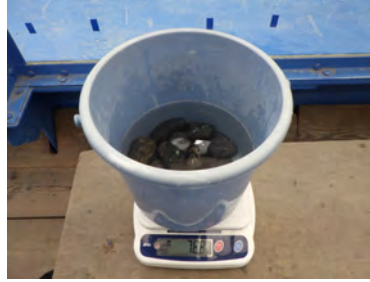
(e) A bucket filled with boulders and water is weighed.
