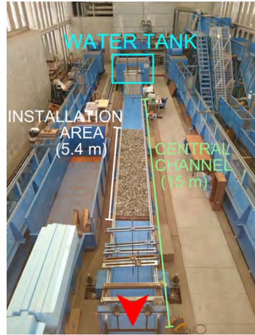
Figure 1: Aerial view of the experimental channel (red arrow for flow direction).
