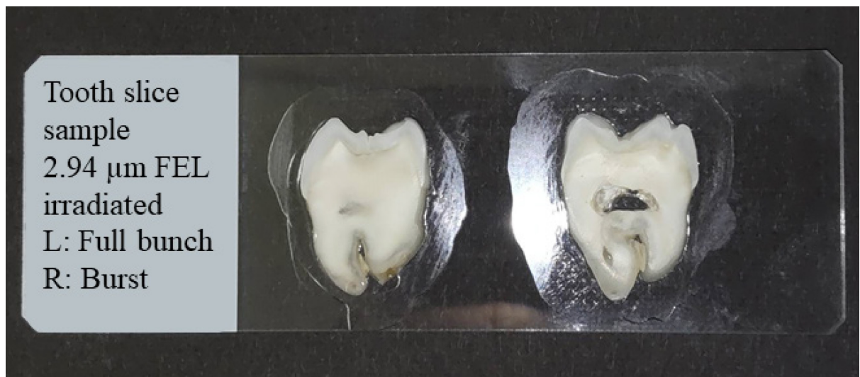
Figure 1 Photograph of tooth sliced to 0.5 mm and attached to the glass slide.
