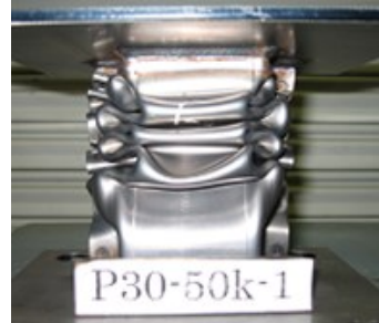
(a) Specimen before crushing (b) Specimen after crushing
