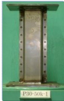
(a) Specimen before crushing (b) Specimen after crushing
