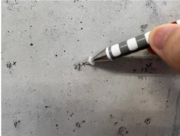
Figure 5.13 Pencil lead breaks.
