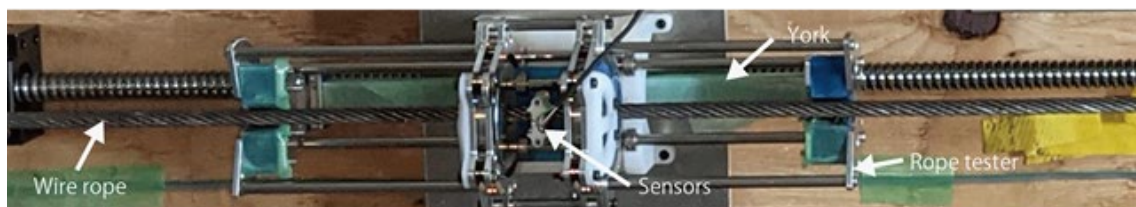
Fig.3-3 View of the rope tester attached to the wire rope during the experiment.
