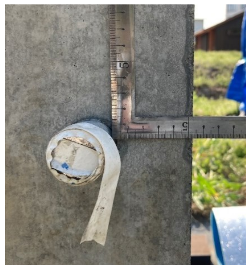
(b) Specimen_3 : \phi_s=33.0\text{mm}
