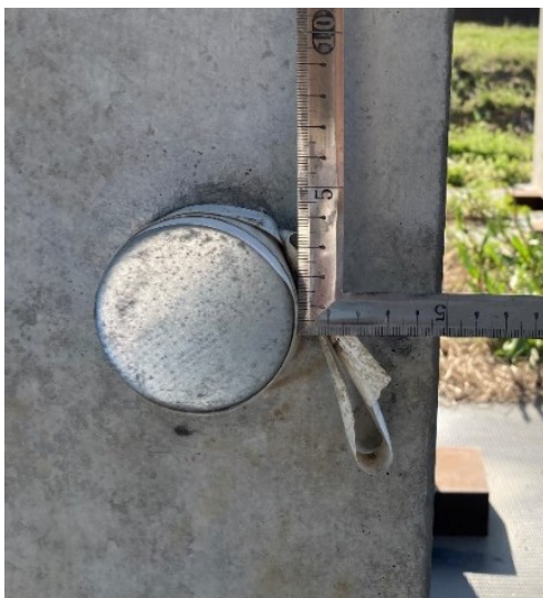
(a) Specimen_1 : \phi_s=63.0\text{mm}
