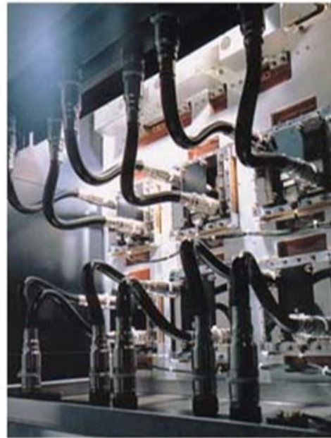
Fig.1-3 Multi-chip module with water cooling cold plate (Hitachi M880, 1990) [4]
