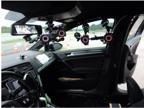
Fig. 6.43 Check motion captures working on test course
