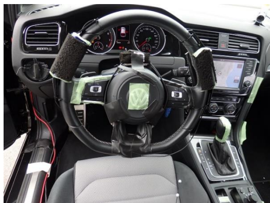
Fig. 6.35 Wheel torque sensor Installation
