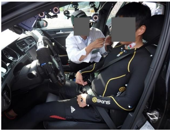
Fig. 6.39 Installation of body markers
