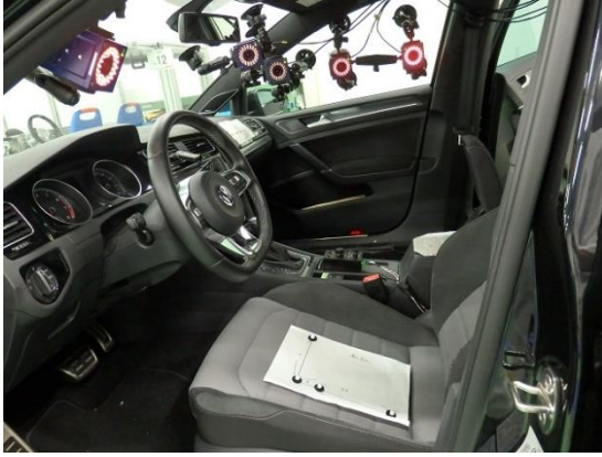
Fig. 6.37 Installation of motion capture cameras
