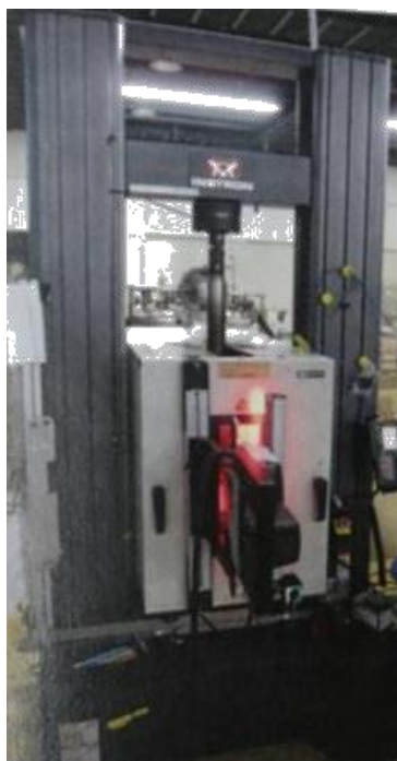
Fig. 2-19 Appearance of high temperature tensile test
