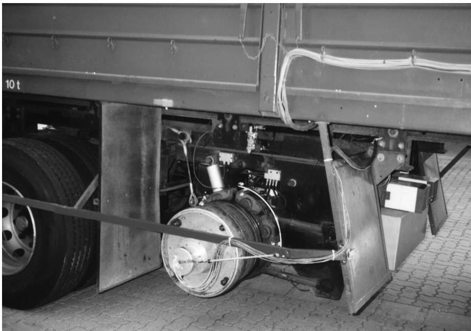
図 2-10 Trailer Type Tire Test Facility (IPW)
