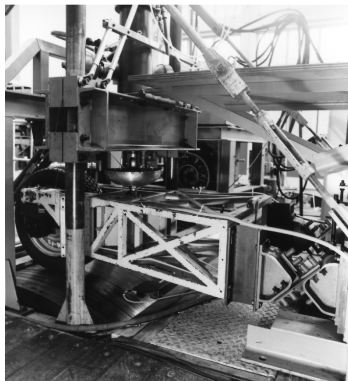
図 5-4 Tire Test Facility on Drum
