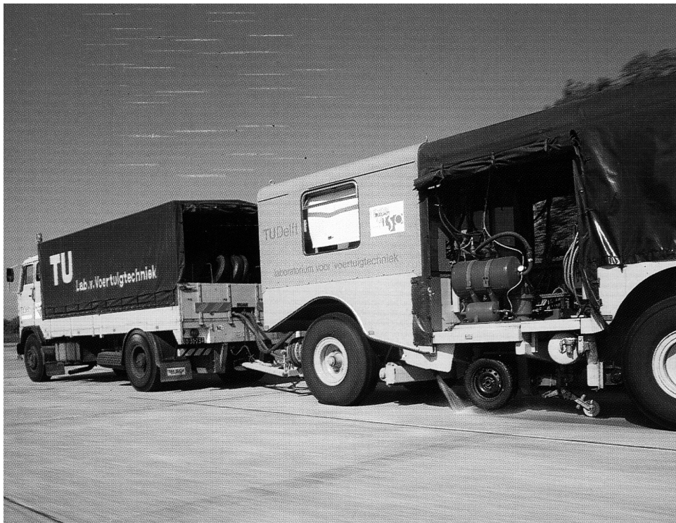
図 2-9 Trailer Type Tire Test Facility (TNO)
