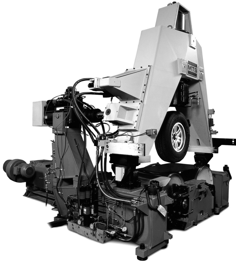
図 2-8 Flat-belt Type Tire Test Facility (MTS)
