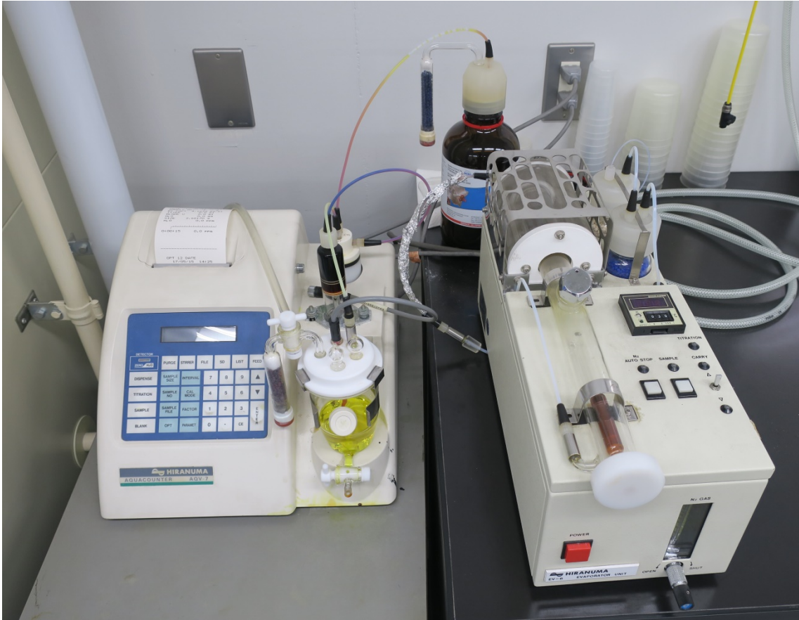
Fig.5.3 Measurement of water content by Karl Fischer method.
