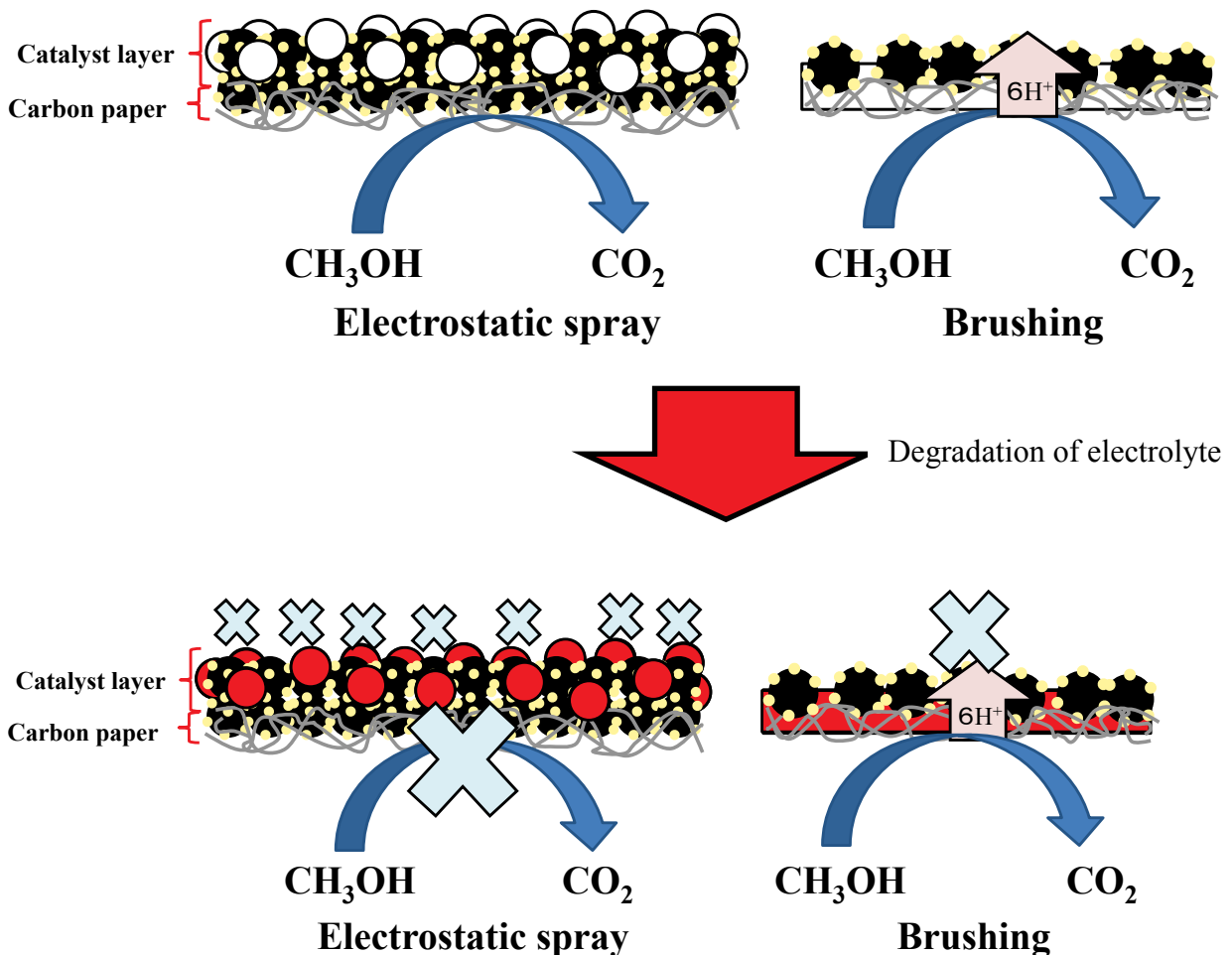
Fig.5-8 Discrepancy of increasing impedance by catalyst layer structure
