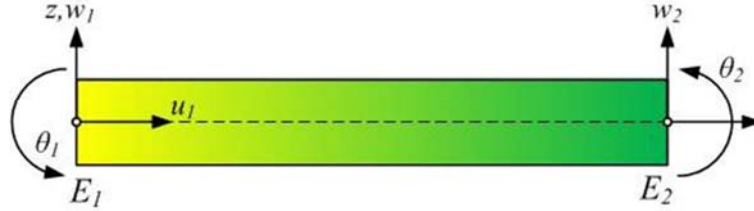
Figure 2.8: Two-node-six-degrees-of-freedom beam element
