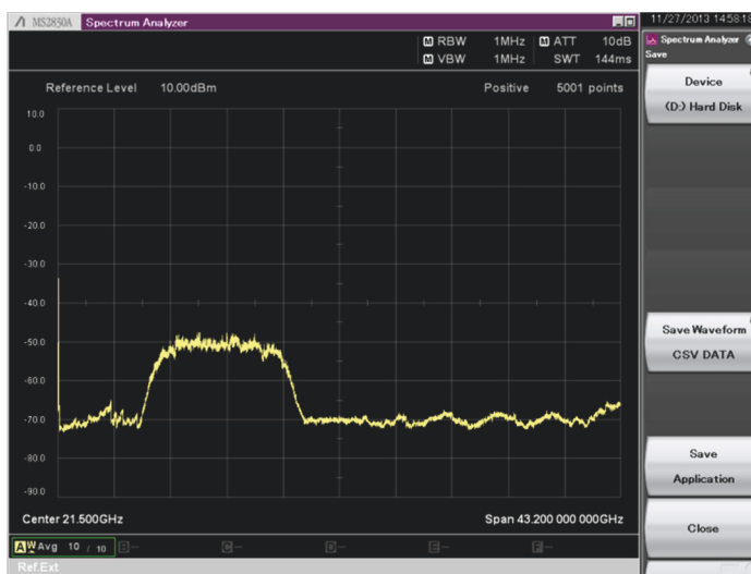
Fig. 6-22 QPSK Modulated signal output from AWG.
