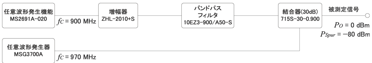
Fig. 4-18 Block diagram of the Test signal generation.
