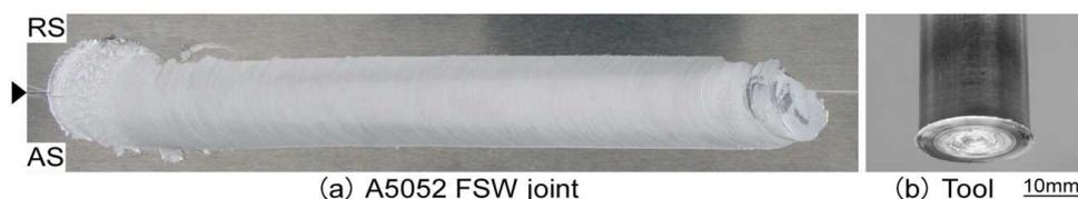
Fig.4.1 Appearances of joint and tool after welding.
