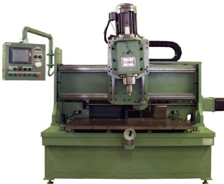
Fig.3.2 Photograph of type FN-II FSW machine.
