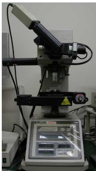
Fig.3.5 Photograph of micro-Vickers hardness tester.
