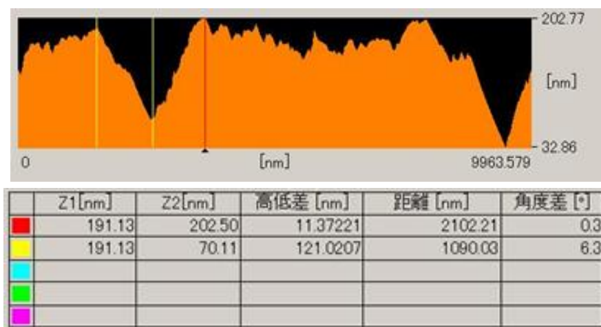
Fig.2-23 Cross-sectional outer surface of Accurel by scanning probe microscope
