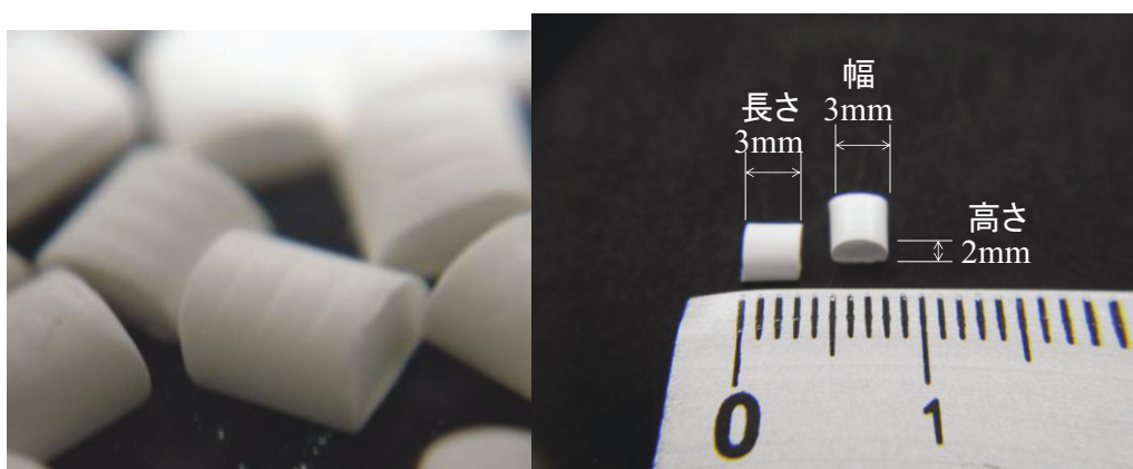
Fig.2-2 Photographs of original Accurel. The true shape of the original Accurel was similar to a half cylinder.
