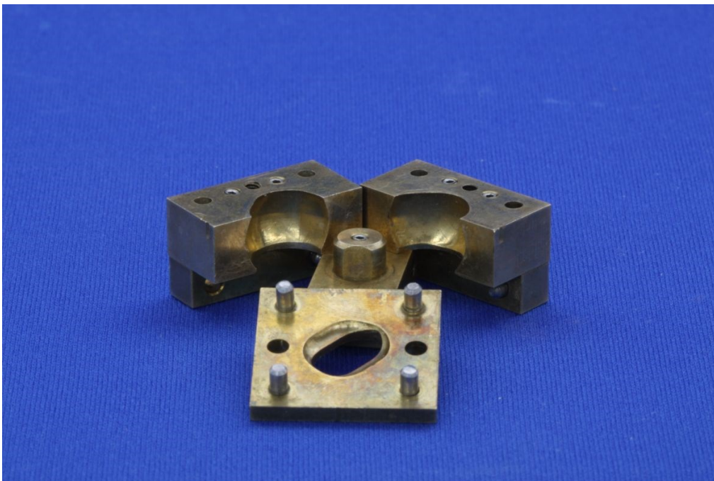
Fig. 2. A photograph of the index used to standardize the dimensions of restorations.
