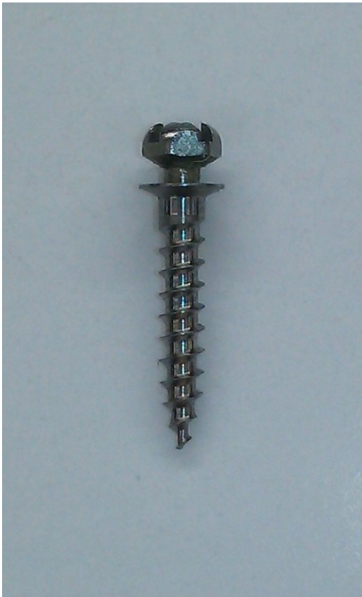
Figure 1. An anchor screw 1.6 mm in diameter and 8.0 mm in length was used.
