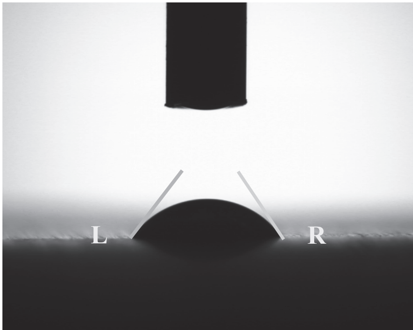
Fig. 1 Drop Master DM500 apparatus fitted with a charge-coupled device camera (a) allowing automatic measurements of the contact angles to be made (b).
