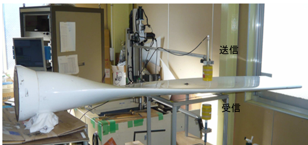
Figure 2-8 Air coupled ultrasonic inspection test system
