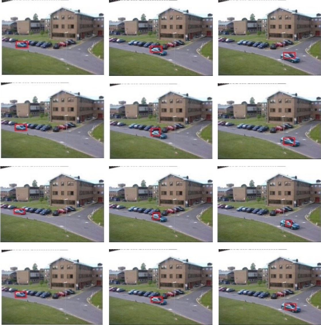
Figure 4.11 Tracking results of sequence V1 as it undergoes scale changes and clutter. Rows 1, 2, 3 and 4 correspond to Mean shift, Color-PF, SIFT-PF, and our tracker, respectively.
