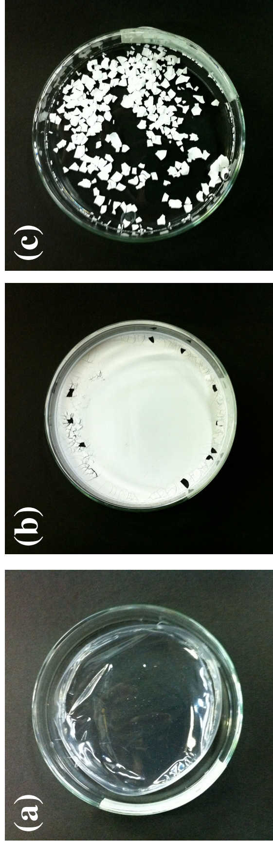
Fig. 3 Appearance of (a) mix-PLA(CHL), (b) mix-PLA(ACN) and (c) mix-PLA(THF) cast films prepared with different cast-solvents.
